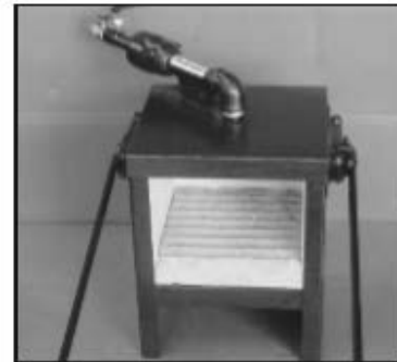
Clarke Pro Branding Fire Box. Larger opening than most forges to allow placement of branding iron.
